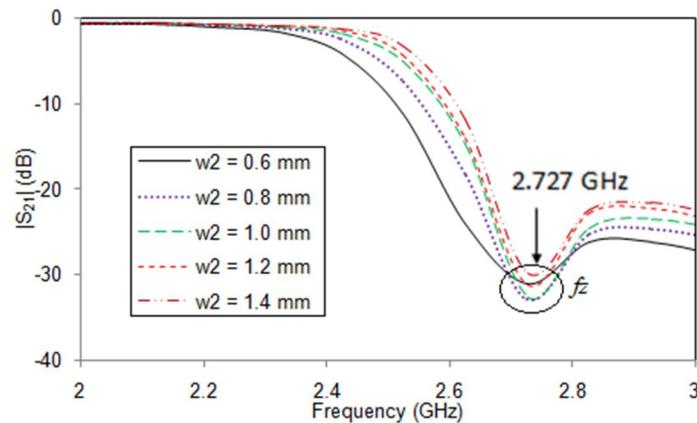
Figure 6. Simulated  $|S_{21}|$  characteristics of the compact filter as a function of width,  $w_2$  of HIML
