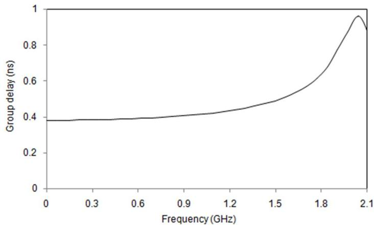
Figure 10. Measured group delay characteristics of the compact lowpass filter with modified PPR
