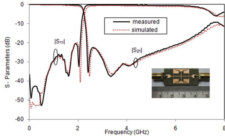
Figure 9. Measured and simulated results of compact lowpass filter with modified PPR
