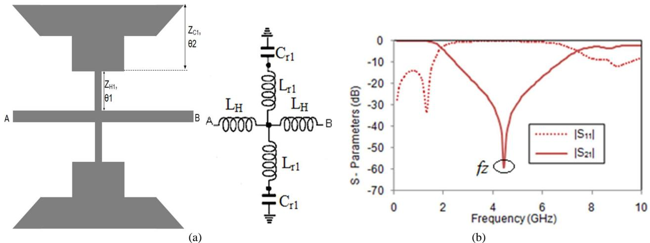
Figure 2. Layout, L-C equivalent circuit and simulated S- parameter characteristics of proposed PPR
