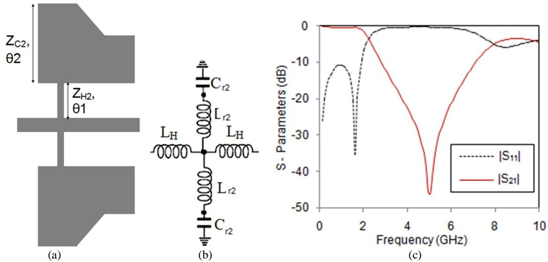
Figure 3. Layout, LC equivalent circuit and response characteristics of MRPR
