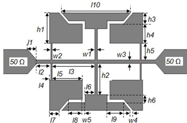
Figure 7. Layout of compact lowpass filter modified PPR
