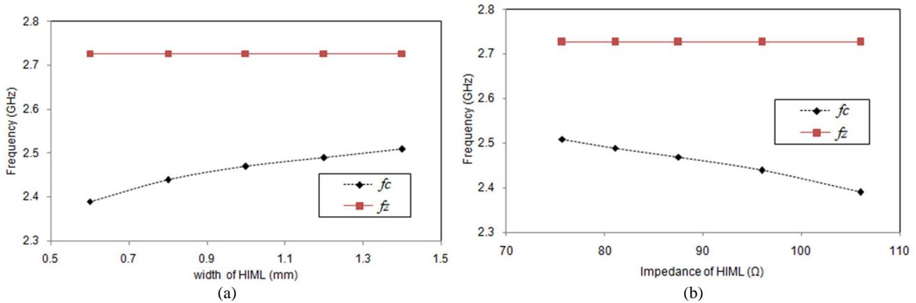
Figure 5. The effect of width of HIML  $w_2$  and characteristic impedance  $Z_C$  on 3 dB cutoff frequency,  $f_c$  and first transmission zero frequency,  $f_z$  of the filter, (a) effect of width of HIML  $w_2$ , (b) effect of characteristic impedance  $Z_C$
