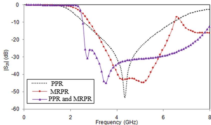
Figure 4. Simulated transmission characteristics as a function of resonators
