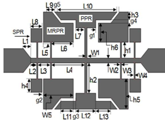
Figure 1. The layout of the proposed filter
