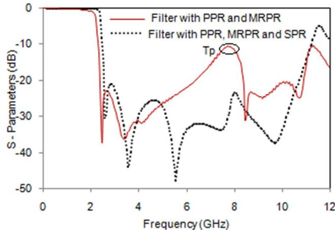
Figure 11. The simulated S-Parameter characteristics of proposed lowpass filter with and without SPRs
