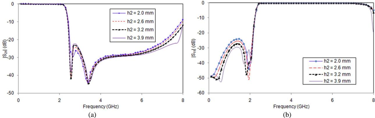
Figure 8 Characteristics of filter as a function of stub height of PPR,  $h_2$ , (a) Transmission characteristics, (b) Reflection characteristics
